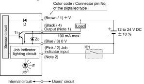
Symbols ... D : Reserve supply polarity protection diode Zo: Surge absorption zener diode
